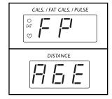
walking belt is moving when the FITNESS PROGRAM button is pressed, the walking belt will slow to a stop. In addition, if the incline of the treadmill is higher than 1%, it will automatically decrease to 1%.
